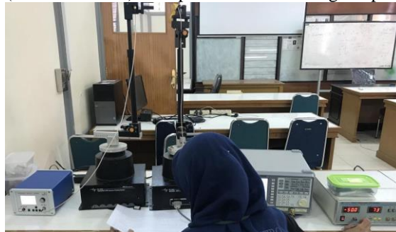
Figure 7. Manual measurement of antenna polarization
