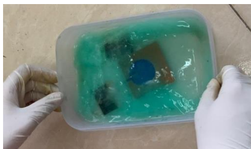
Figure 5. Antenna dissolving process
