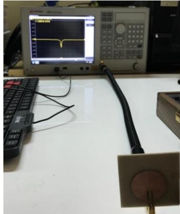
Figure 6. Antenna Measurement using Network Analyzer
