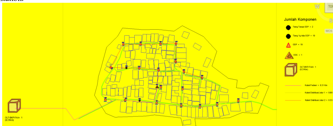
Figure 5. FTTH Network Routing Design
