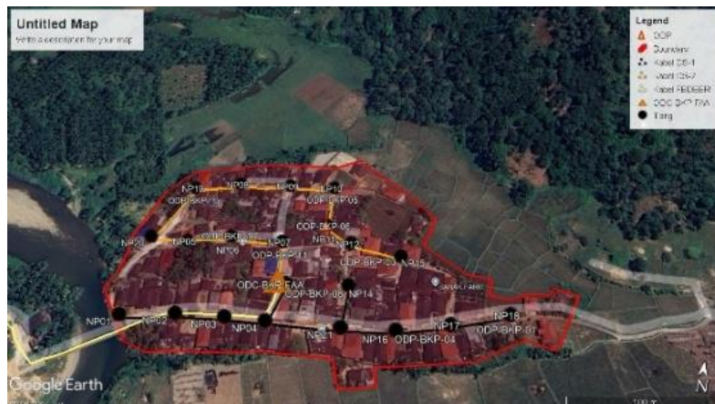
Figure 4. Locations of Devices and Fiber Optic Cable Routes
