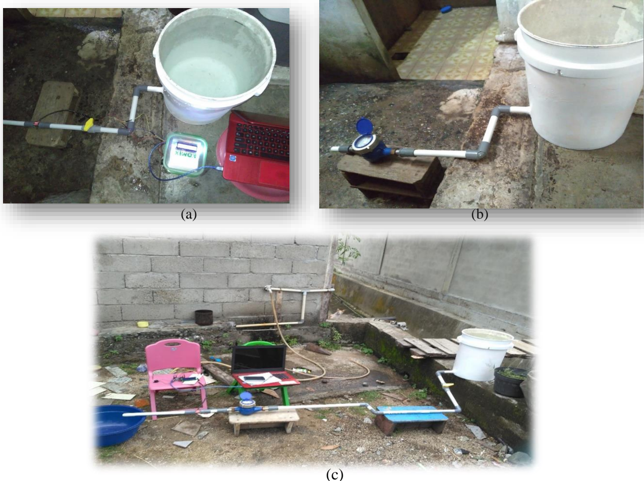
Figure 4. Assembling the Equipment using a Flowmeter
